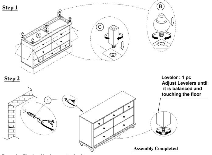
Remark: Tipping Hardware attached to the back stretcher
