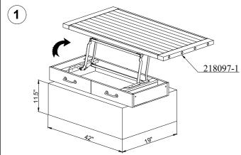
SHOWN ARE THE RECOMMENDED TOP SUPPORT DIMENSIONS FOR EASE OF LEG ASSEMBLY.
