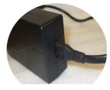
Check power cord for damage and connection to transformer. If power cord has no damage and its connection to transformer is good and green light is not on, then replace transformer.
