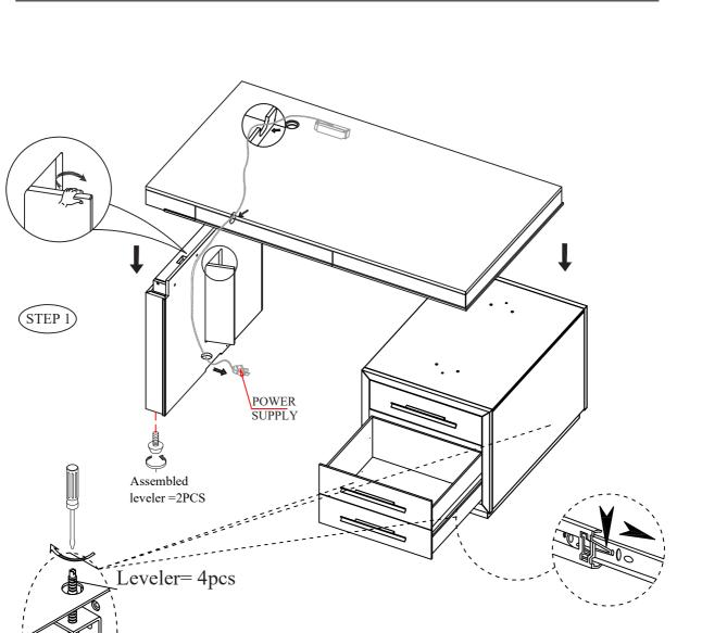
To adjust and access levelers, first remove plastic cap if it have with a flat-head screwdriver. Using the same screwdriver, proceed to turn leveler clockwise to raise the piece, or counterclockwise to lower the piece.
