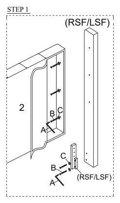
DO NOT TIGHTEN ALL THE BOLTS UNTIL COMPLETELY ASSEMBLED
